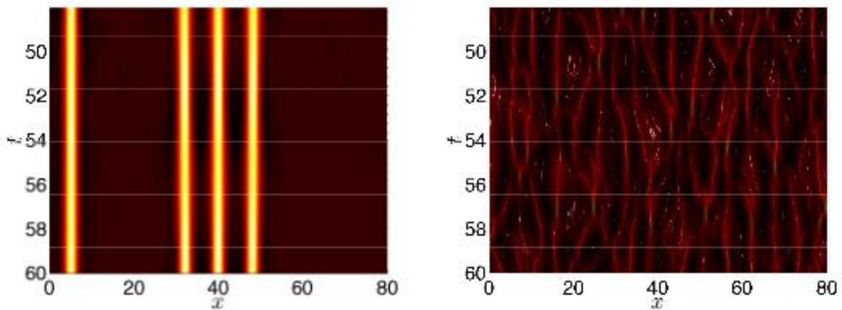
**Fig. 17** Hovmöller diagram of  $|Q(x,t)|$  for regular dynamics with  $\varepsilon = 0.095$  (left) and chaotic dynamics with  $\varepsilon = 0.2$  (right) for the driven and damped Schrödinger equation (15).
