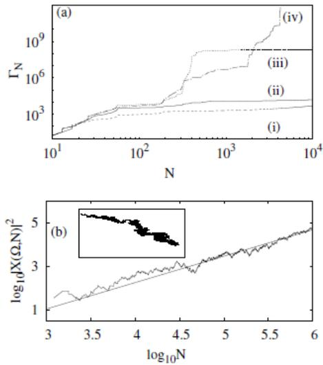
FIG. 3. (a) Phase sensitivity exponent  $\Gamma_N$  versus  $N$  showing (i) torus for  $A=0.3111$ , (ii) wrinkled torus for  $A=0.3112$ , (iii) SNA for  $A=0.311227$  and (iv) chaos for  $A=0.31124$ . (b) Finite-time Fourier spectrum  $|X(\Omega, N)|^2$  vs  $N$  on logarithmic scale for SNA for  $A=0.311227$  with the exponent  $\beta = 1.21$ . The inset (b) shows fractal walk in the complex plane ( $ReX, ImX$ ) for the SNA attractor.
